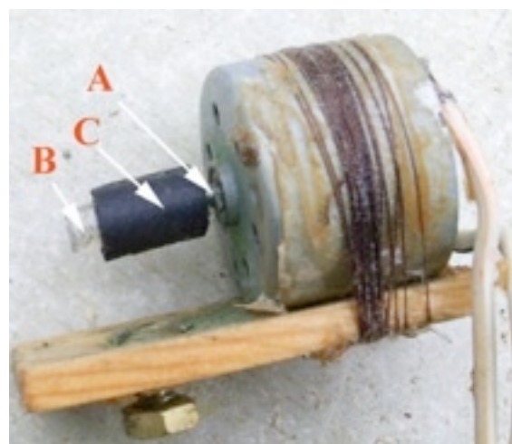
A - Axle of generator B - Piece of plastic tube on axle C - Rubber tube cut from the connection of a bicycle pump
